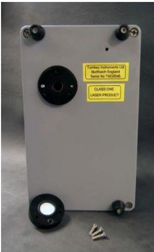
Turnkey's monitors require a flow and filter check every 3 months (later models have an inbuilt flow stabiliser, consult technical support if unsure). This is a simple procedure, which can be easily carried out following the Turnkey filter change flow chart.
