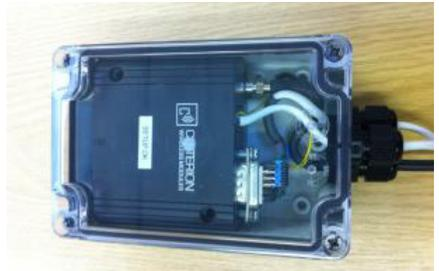
*Remote GSM modem – Dust monitor end.*
